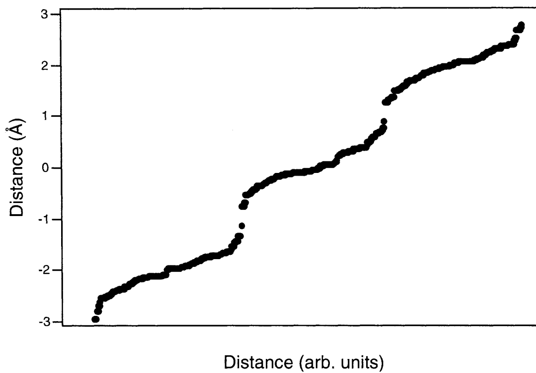
Figure 21: Predicted step heights for Al-Ni-Co oriented to the (0, \bar{1}, \bar{1}, 0, 1) plane.
